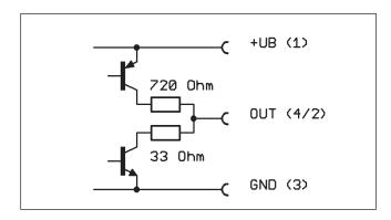
The output drivers are asymmetrical push pull output stages with the protective resistors of 720  $\Omega$  and 33  $\Omega$  as shown.
